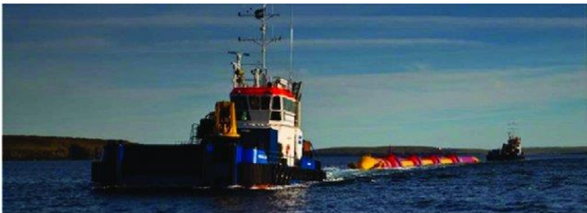
Figure 6.1 A Pelamis P2 device being towed for installation at EMEC in 2012 (Pelamis Wave Power) (Gray, Dickens, Bruceclan, Ashton, & Johanning, 2017)
