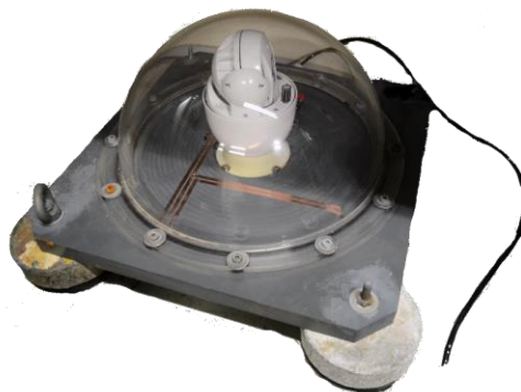
Figure 2-13: Underwater video camera used in the experiments
