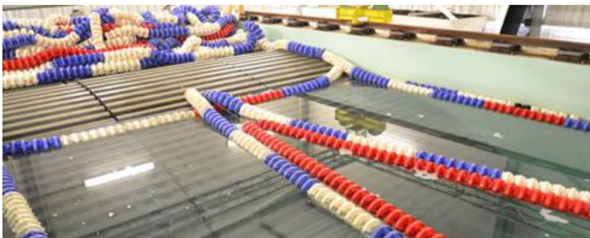
Figure 2-3: Tank beach and swim lines for wave absorption
