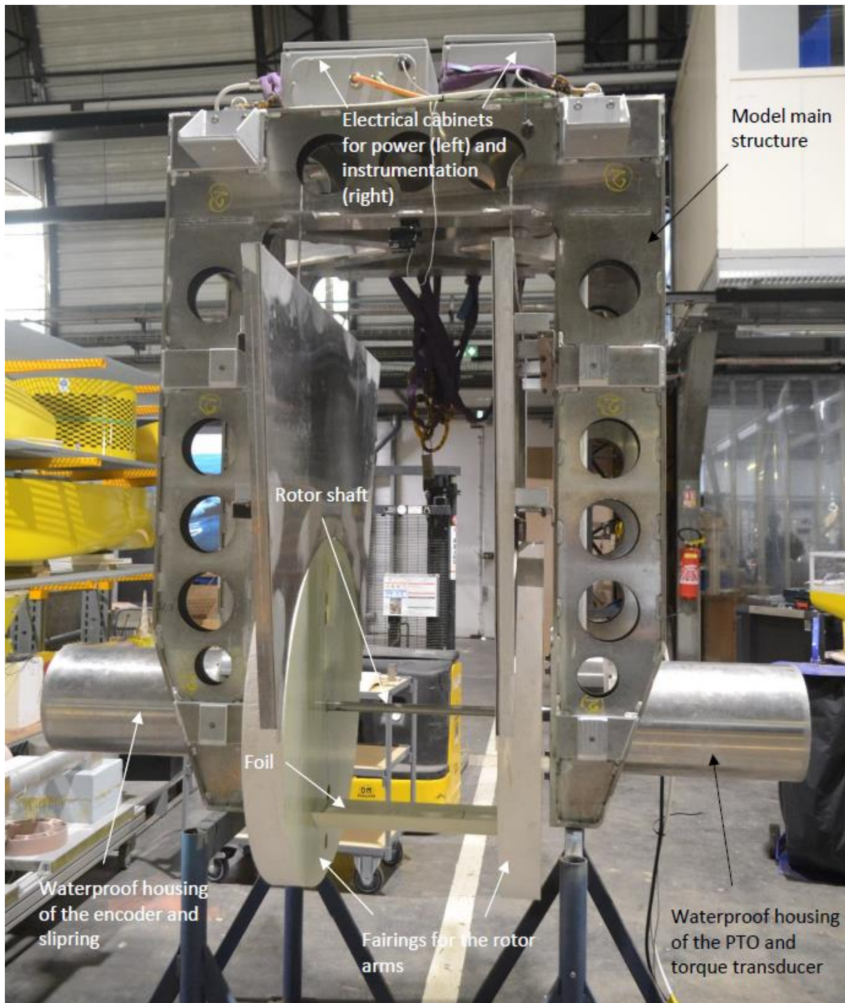
Figure 2-5: Overview of the rotor and support structure
