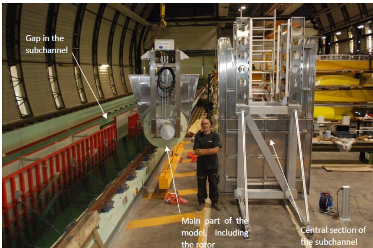
Figure 2-4: Overview of the model structural elements
