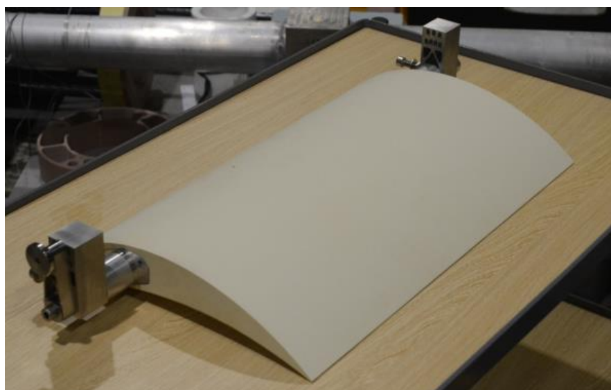
Figure 9: Curved foam foil used during campaign, including strut connectors which are later embedded in the foam fairings. Courtesy of ECN.
