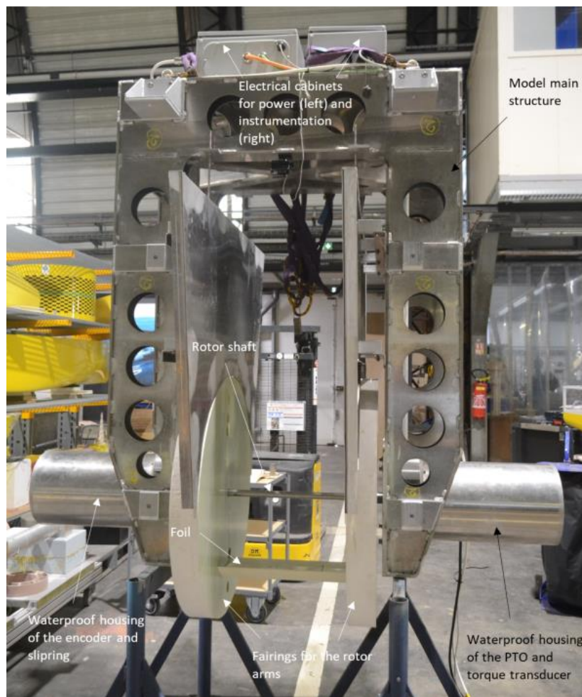
Figure 8: Removable aluminium rotor top structure with rotor fairings and housing for torque transducer and encoder. Courtesy of ECN.
